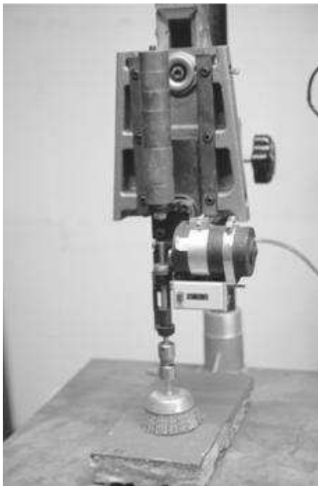
Fig. 10 Apparatus to test the resistance against abrasion
