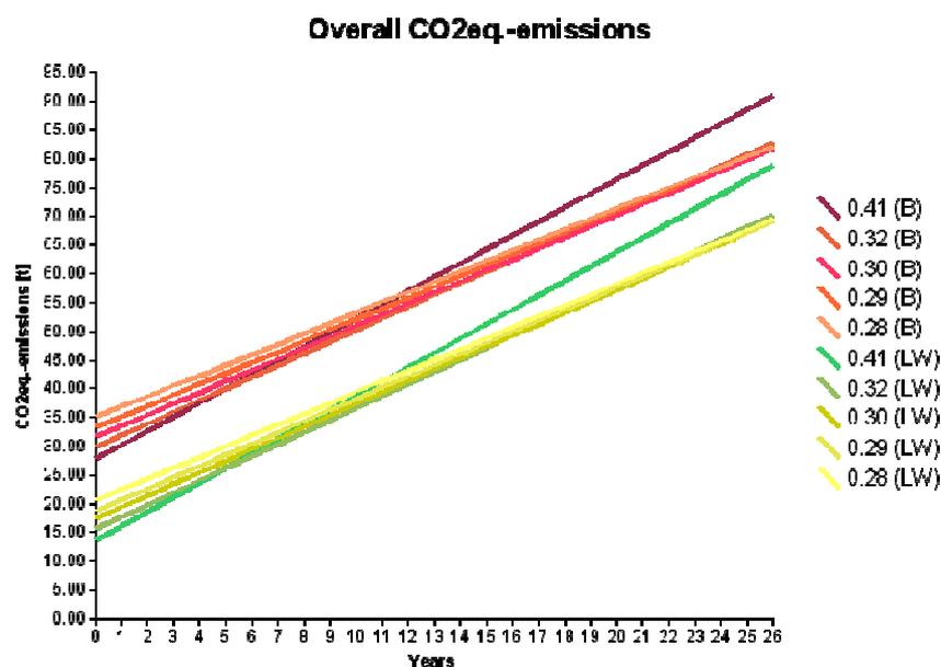
**Fig. 8** Diagram 3: The CO<sub>2</sub>-emissions due to manufacturing and operation of the case study house calculated in dependence on time for both the heavy (B – brick house) and the lightweight (LW) modifications of the building envelope (represented by the mean U-values).
