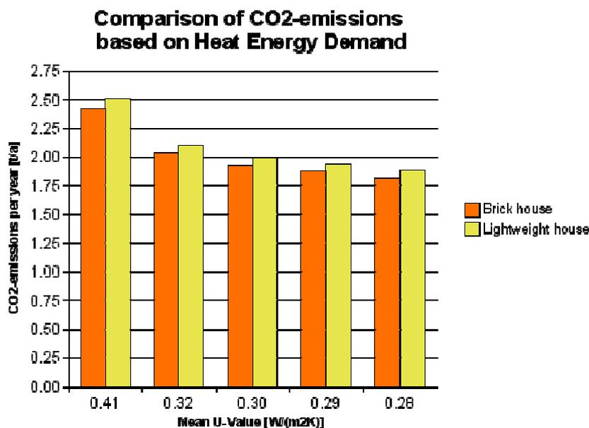
Fig. 6 Diagram 1: Comparison of the CO<sub>2</sub>-emissions based on energy demand for heating against the mean U-value of the heavy (“brick house”) and lightweight variant of the building envelope.
