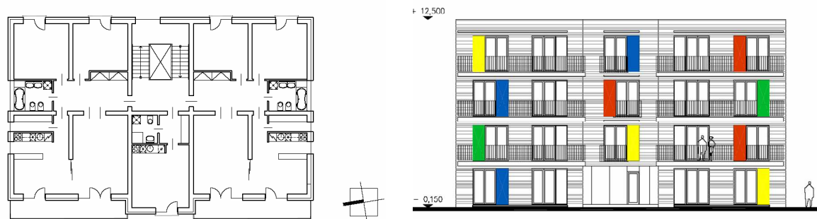
Fig. 1 Four-storey residential building – typical floor and entrance facade
