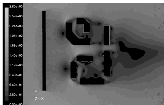
Fig. 6 Wind flow patterns around buildings with acoustic screen Fig. 7 Wind flow patterns around buildings with earth berm
