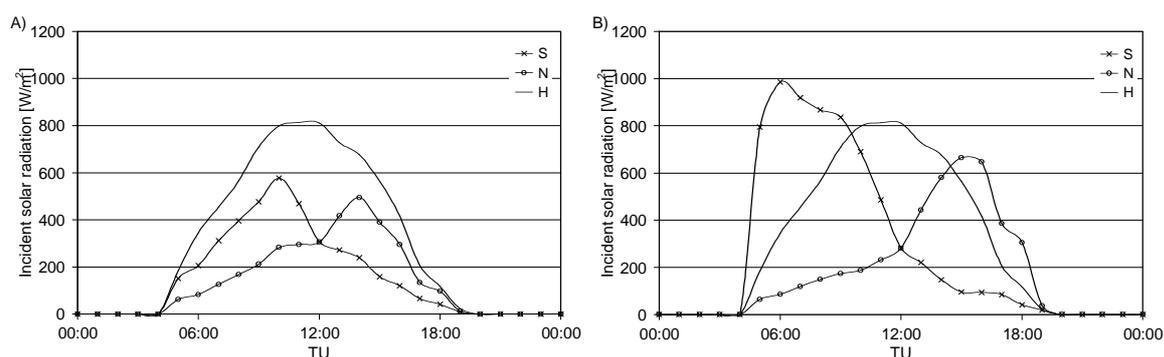
**Fig. 2** Incident solar radiation: A) building in a street canyon, B) detached building
