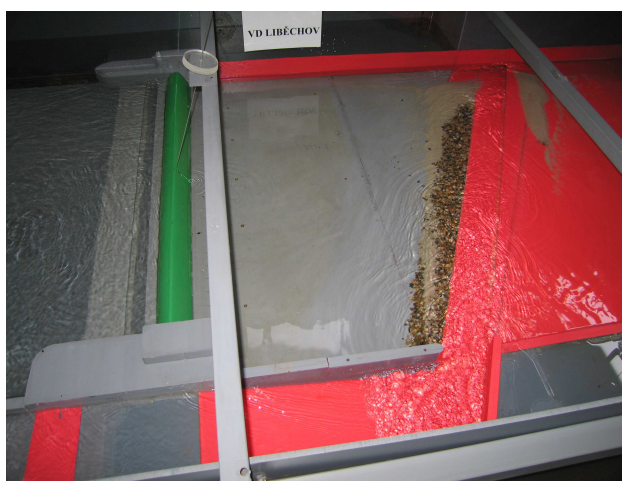
Fig. 2 Test.6 – successful washing away of the suspended load.
