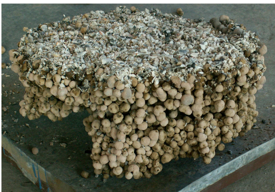
Fig. 3 Burned aggregate right under the ignition layer
