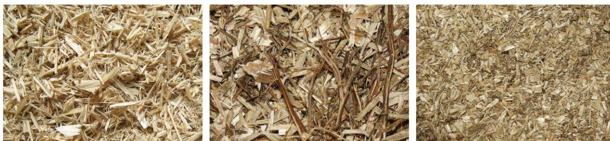
**Fig. 1** Wood particles used in cement bonded particleboards
