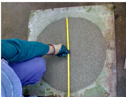
Fig. 1 Measuring of rheological properties at the building site (Slump Flow test)
