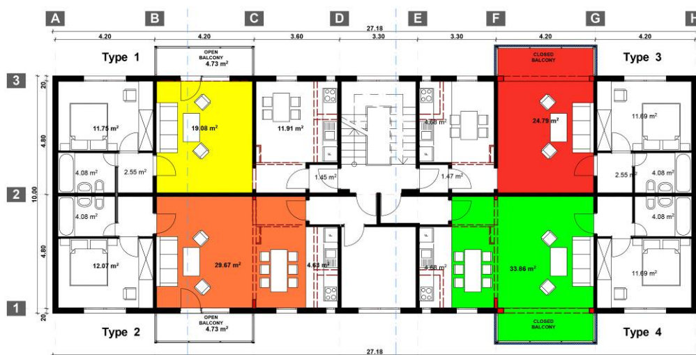
Fig. 5 Horizontal reconfiguration and optimization of usable area in apartments
