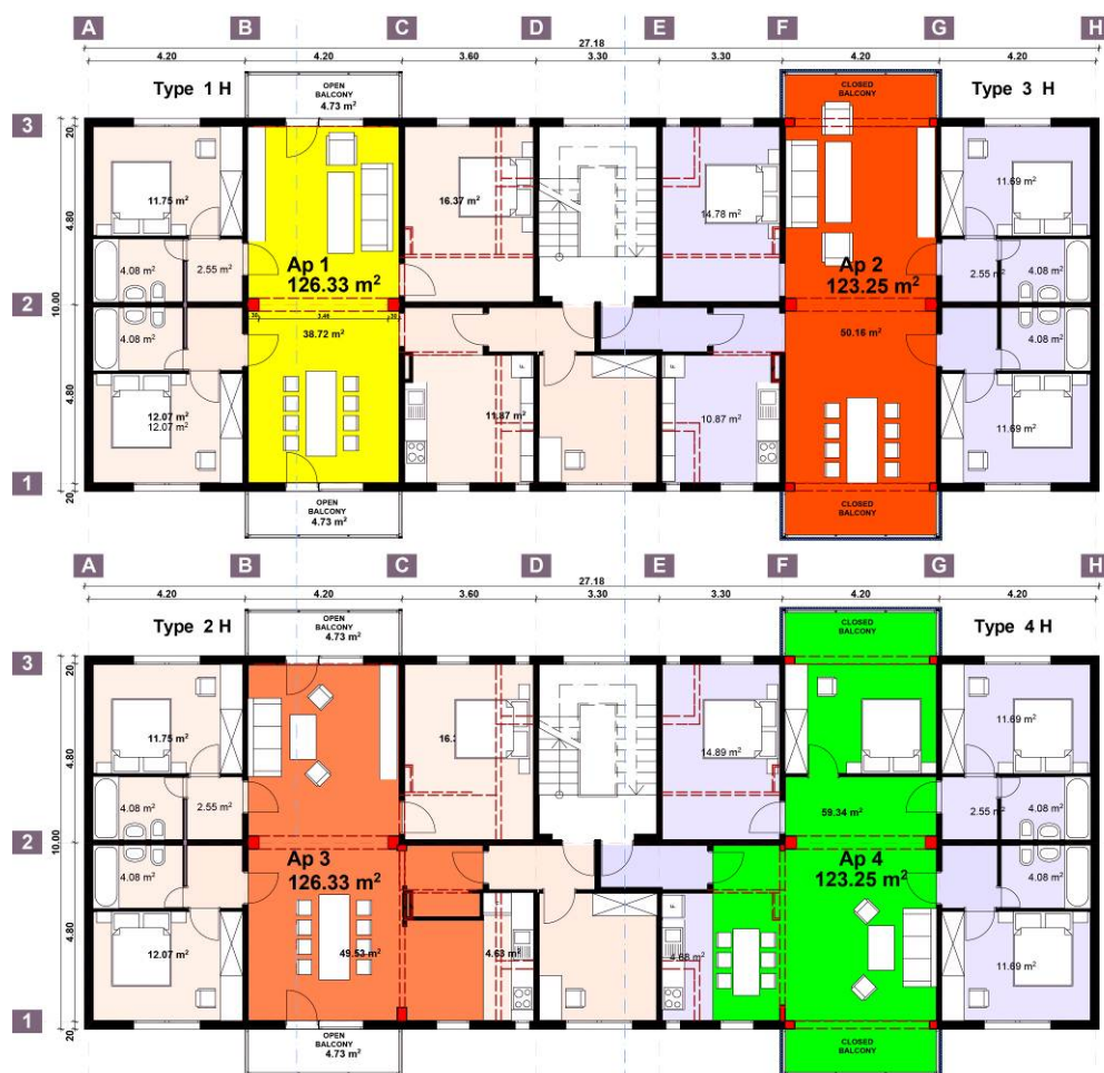
Fig. 6 Horizontal reconfiguration by coupling two apartments
