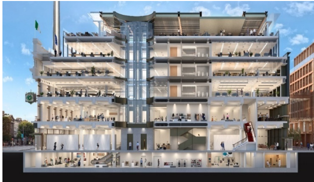
Fig. 6 Rendered cross-section of the refurbished Clerys Department Store showing the increased structural grid of the upper storeys and terraced extension. (© Visual Lab)
